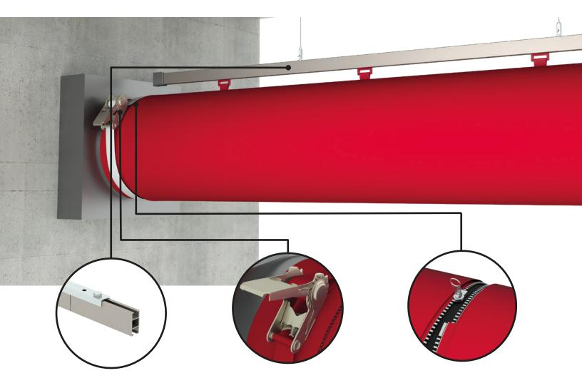
Ducts are suspended with Adjustable Cable Drop. The H-rail, so named because it looks like a H in the cross section, is made out of anodized aluminum, making it an excellent choice for corrosive environments.
